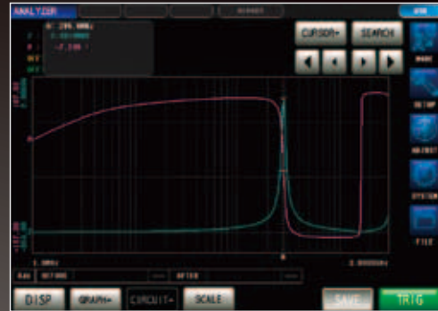
High-stability, high-speed sweeping measurement up to 3 GHz
